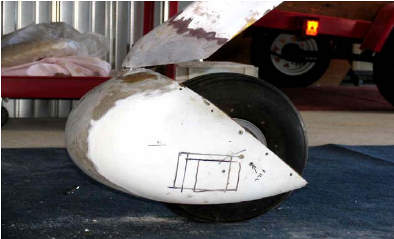
A Nosewheel Pant Being Fitted
