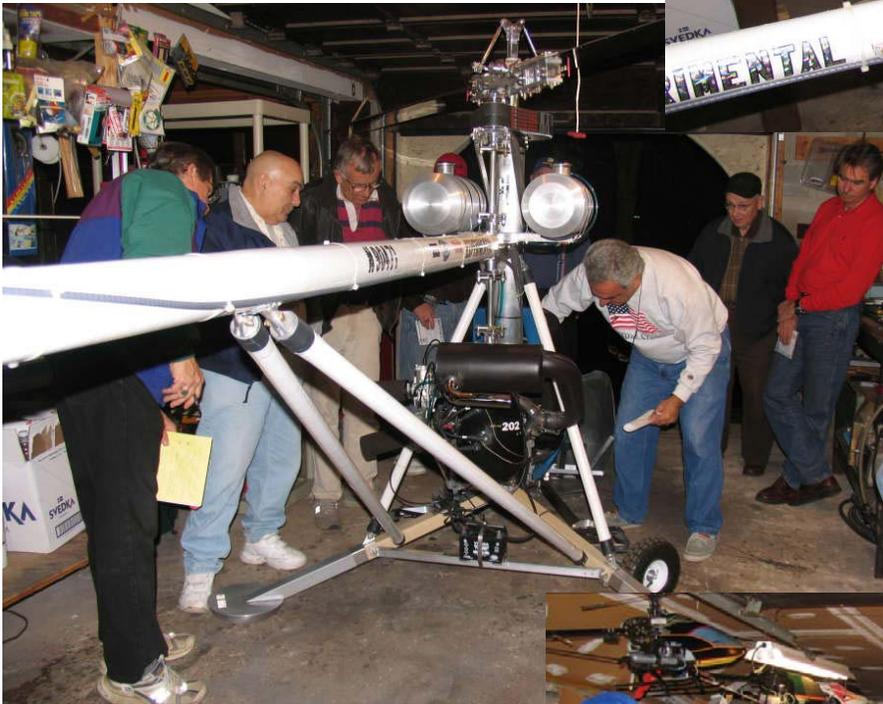
power to the secondary reduction at the top of the mast which then drives the main rotor through a second high capacity HTD cog belt."
