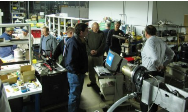
The top picture is of the "R&D" area at IPS and features their new brushless generator for aircraft applications. Very large capacity generators have never been feasible due to problems with accelerated brush wear from high currents required and the need to have the units survive to a reasonable TBO.
